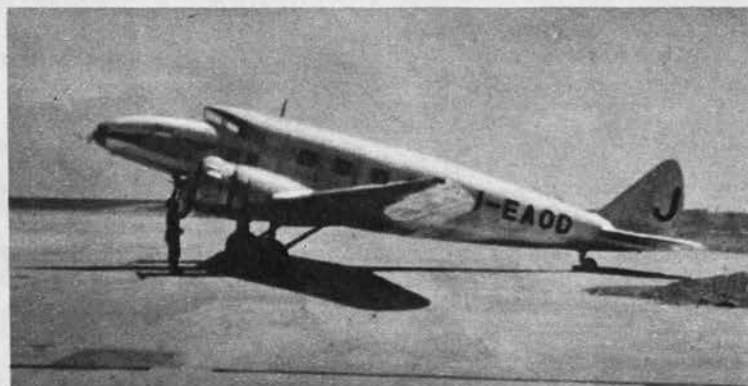
Thora, a prewar commercial plane, is strictly Jap design. Nose is pointed; small fin has sharply slanted leading edge much like Dinah's.
